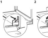
Open the door fully and hold the two door hinges.
