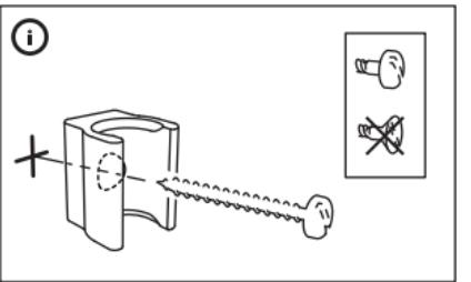
**GB** As wall materials vary, screws for fixing to wall are not included. For advice on suitable screw systems, contact your local specialised dealer.
